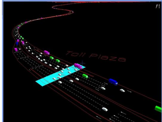
ILTP consulting Transport Planners were commissioned by Hyder, Consulting Engineers to undertake a capacity assessment of the Dublin Port Tunnel (DPT) using the Paramics Microsimulation Model. The brief was " to identify the level of traffic that will maintain an acceptable level of service such that congestion and queuing do not occur in the tunnel"
